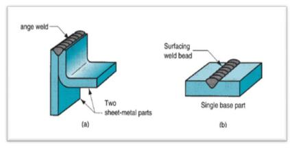
Figure 7 (a) Flange welds and (b) surfacing welds
