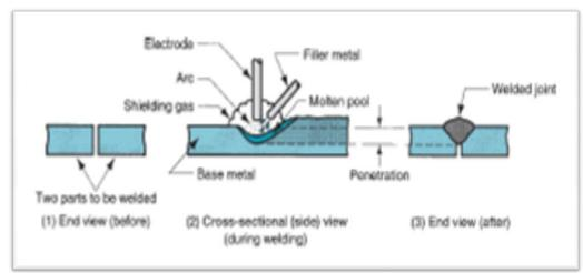
**Figure 1** Basics of arc welding: (1) before the weld; (2) during the weld (the base metal is melted and filler metal is added to the molten pool); and (3) the completed weldment. There are many variations of the arc-welding process.
