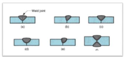
**Figure 4** Some typical groove welds (a) square groove weld, one side; (b) single bevel groove weld; (c) single V-groove weld; (d) single U-groove weld; (e) single J-groove weld; (f) double V-groove weld for thicker sections. Dashed lines show the original part edges.
